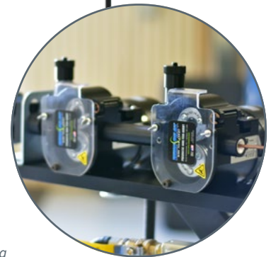
Tandem PFA-LM Wire Feed Assists installed on a Turn Table for Large Wire Dispensing
