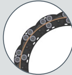
Internal view showing path of wire along rollers.
