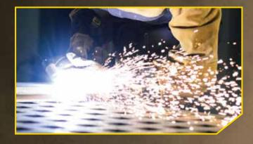
**Long arc stretch** – When you are in an odd position or trying to hit a corner, Cutmaster 60i's extra-long arc will stretch to keep constant contact with the workpiece.
